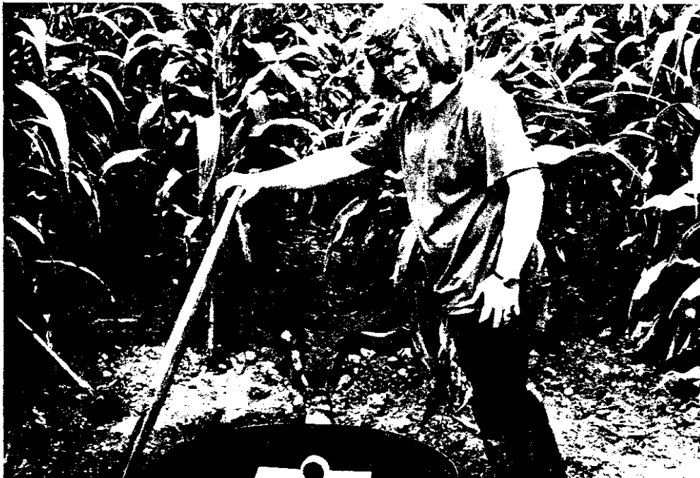
Figure 10-4. Runoff from 3 m X 4 m plots was recorded with a tipping bucket apparatus and an event recorder.
